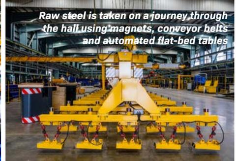
Raw steel is taken on a journey through the hall using magnets, conveyor belts and automated flat-bed tables
