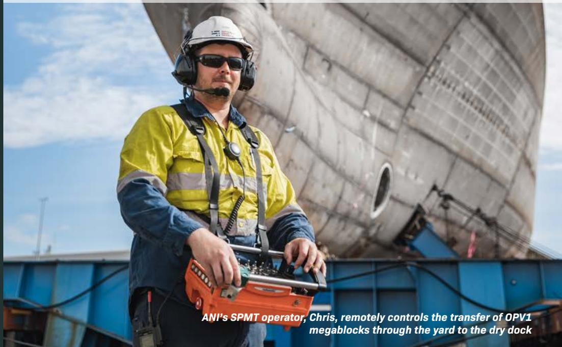
ANI's SPMT operator, Chris, remotely controls the transfer of OPV1 megablocks through the yard to the dry dock
